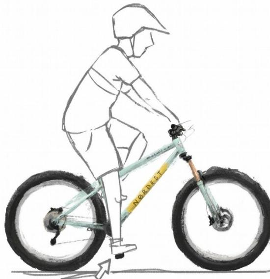
You should also adjust the inclination of the saddle. You will be able to move the extremities of the saddle up and down by using the bolt under the saddle. A common position is to place it in a parallel position to the ground. You can also move the saddle forward and backward sliding it by the rails.
